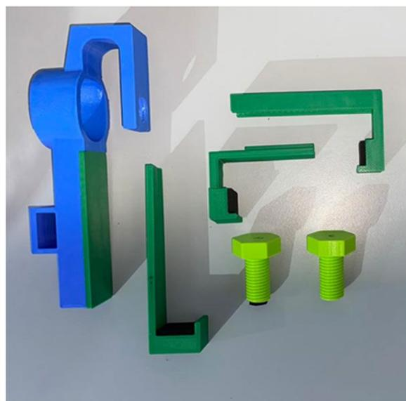
**Fig. 18** Disassembled 3D-printed modified universal adapter
