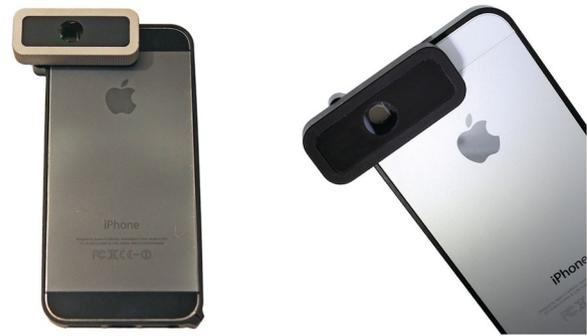
**Fig. 1** D-Eye prototype attached to an iPhone 5 and iPhone 5 s from the left [19]
