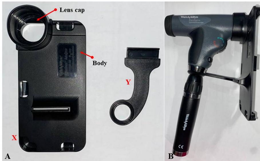
**Fig. 6** Original adapter of PanOptic ophthalmoscope. **a** Main phone holder labelled as X and connector labelled as Y. **b** Assembly of the adapter with the ophthalmoscope
