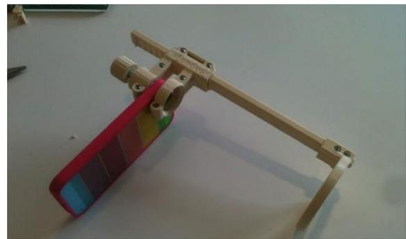
**Fig. 2** 3D-printed retinal image acquisition adapter [20]
